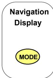
Press the MODE key three times brings up a screen which displays navigation data received from the GPS or other device, eg.
