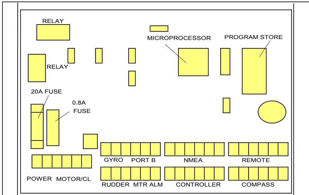
Figure 3.1 Layout of S81.01 Junction Box components and connectors.
