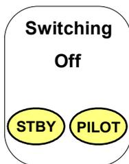
Press the STANDBY and PILOT keys together.
