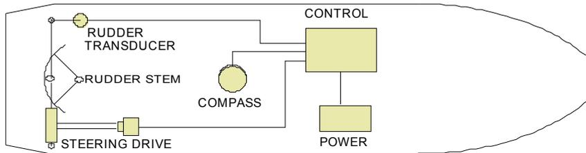
Figure 1.1 Basic components of a marine autopilot.
