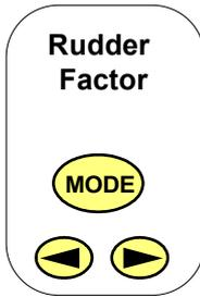
Press MODE twice to adjust the RUDDER FACTOR. This may be increased or reduced using the arrow keys. In the auto-tune mode, this value is the 'starting point' which applied when the pilot key is pressed. As the vessel travels, the effective rudder factor is internally adjusted above or below this point. In the two Manual modes, this setting becomes the fixed rudder factor. There is more about the rudder factor in Sec 2.7.
