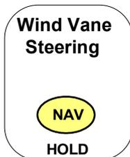
If a wind instrument is fitted, steering to the wind is activated by holding down the NAV key for 2 seconds. When data is being received, the top right display shows the relative wind angle, eg:
