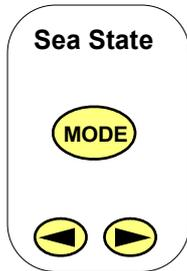
Press the MODE key once. The display shows the current control mode setting.
