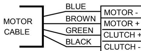
Figure 3.11. Connections to a mechanical steering drive motor.
