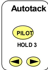
The autotack feature produces a delayed course change which is useful for single handed sailing. Hold the PILOT key down for the beep after the DODGE prompt and the screen shown on the left appears:
