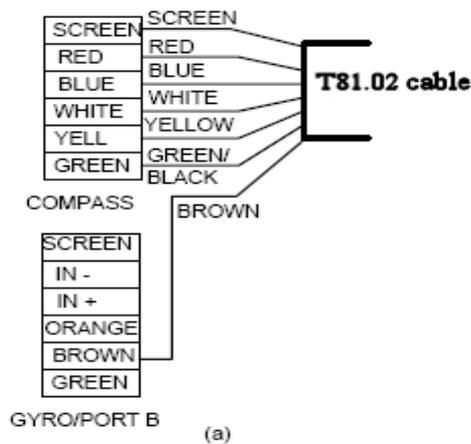
Figure 3.4. Socket connections for the S81.02 compass
