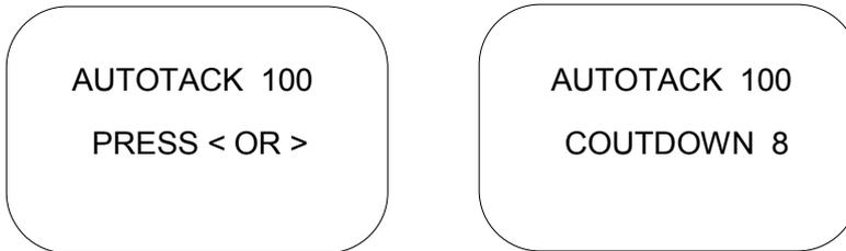
The number on the top line shows the angle through which the vessel will turn. This may be adjusted in the Menu (Sec 2.5).
